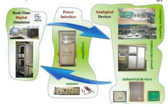
Platform of smart building: The platform is dedicated to the research on smart energy management and auto-consummation. It consists of a demonstrating building with associated measures and instrumentation. The real time management strategy takes into account comfort data, consummation and production and other factors.
