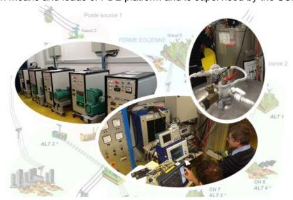
Platform of real time simulation and PHiL: This platform offers the tools for electrical system design, optimization and control. It allows users to actualize researches on all kind of emulated grids with interaction with real components. This modular platform is suitable for different research thematic, from electrical vehicle to renewable energy resources.
