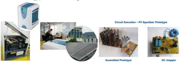
Platform of reconfigurable electrical grid: This platform regroups several real instrumented and flexible electrical grids with a reduced size of 30kVA. It allows the study on different structure of future smart grid. The reconfigurable distribution and industrial grids use the production means and loads of PDE platform and is supervised by the SCADA platform.
