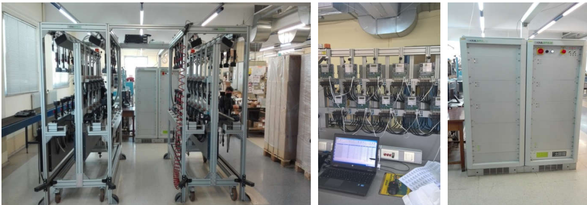
Figure 1: HEDNO Laboratory testing facility for measuring equipment with Iskramatic-CATS Meter Test Station.
