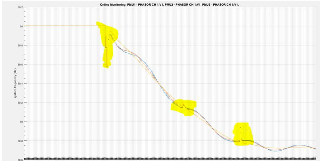
Figure 27 : Indication of UFLS actions observed in the PMU frequency measurements.
