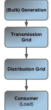
Transmission Grids (e.g., 380 kV, 220 kV, 110 kV) Medium Voltage Distribution Grids (e.g., 10 kV, 20 kV, 30 kV) Low Voltage Distribution Grids (e.g., 0,4 kV)
