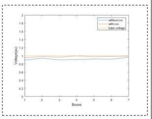
For each condition buses voltage recorded with and without controller. In each case recorded quantities were plotted and compared with base voltage case.
