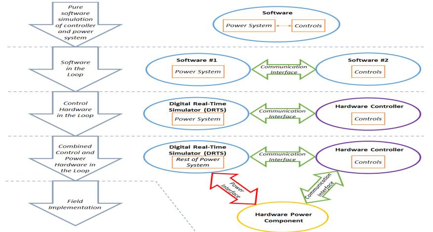
The combination of CHIL and PHIL simulation allows to test a controller in a CHIL configuration, while critical power components are incorporated as physical devices (PHIL simulation) allowing to analyze more realistic real-world based conditions.
