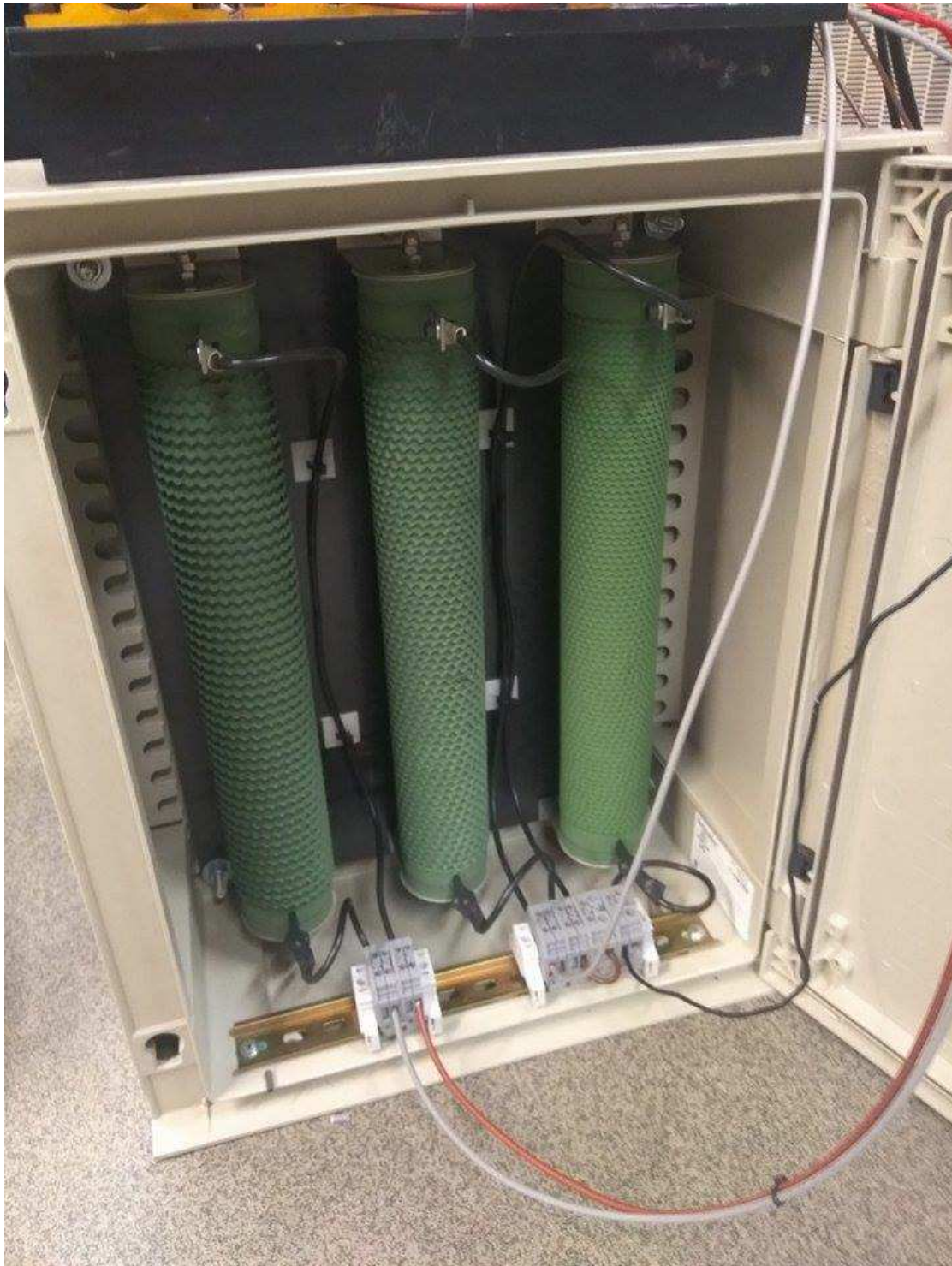
Figure 7: Parallel resistors for the PV emulator
