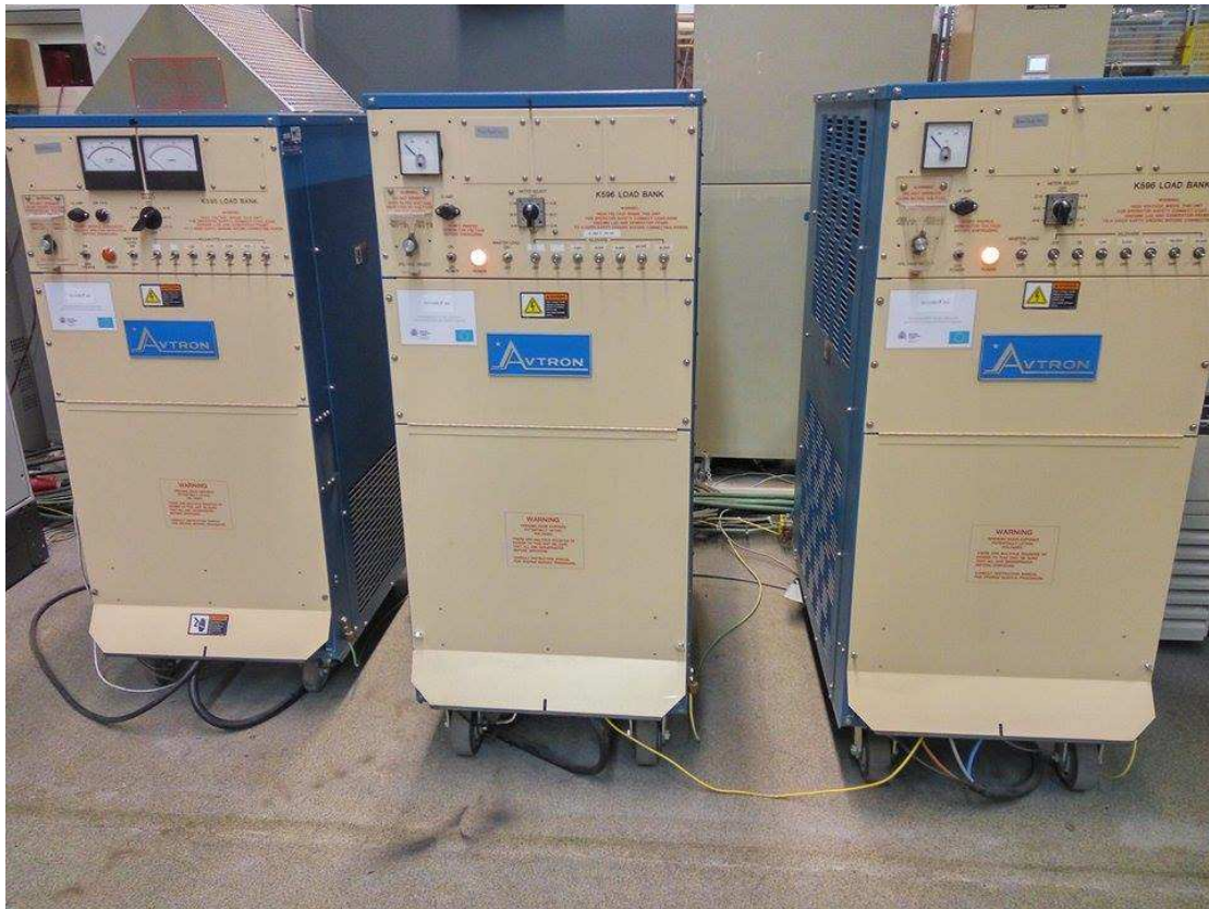
Figure 14: Resistive and inductive load
