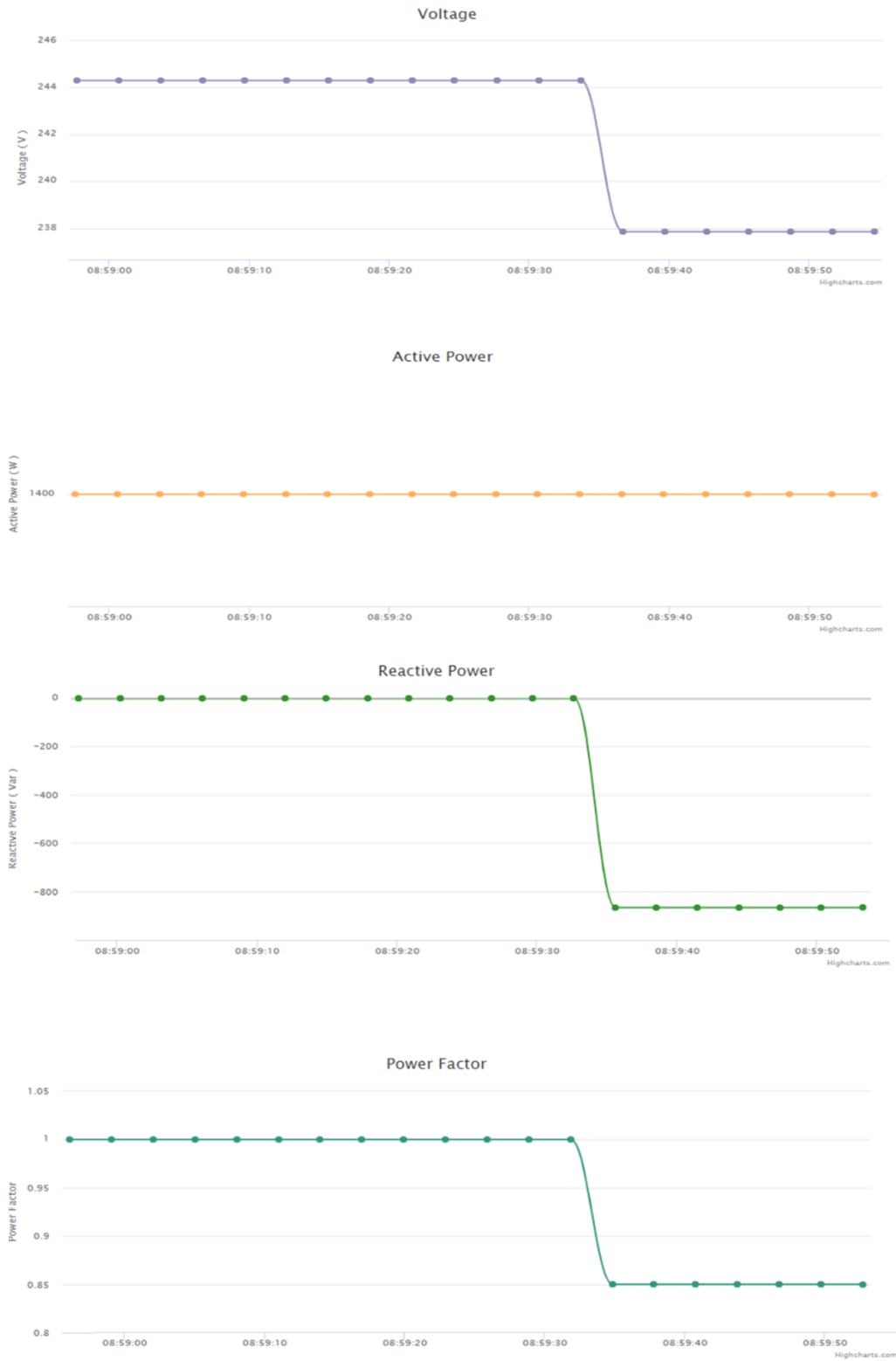
Figure 4: Voltage, active power, reactive power and power factor of the inverter via the GUI of the Virtual Lab
