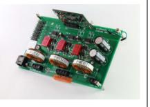
converter systems. The partners in this Transnational Access project are part of this initiative, and they have developed three blocks, namely, DC-DC converter (red board on the left), AC-DC converter (green board on the right) and motherboard.
