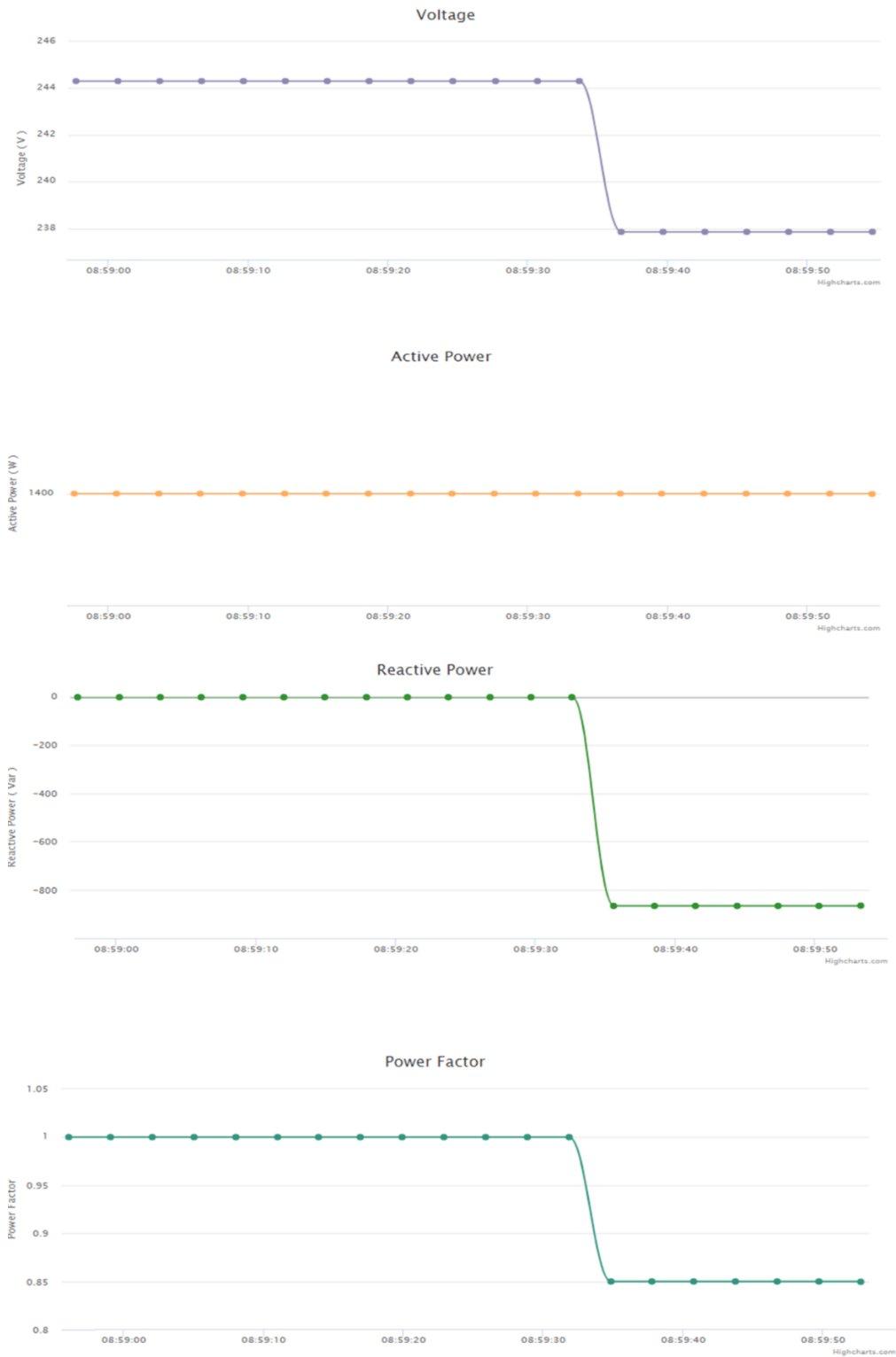
Figure 4: Voltage, active power, reactive power and power factor of the inverter via the GUI
