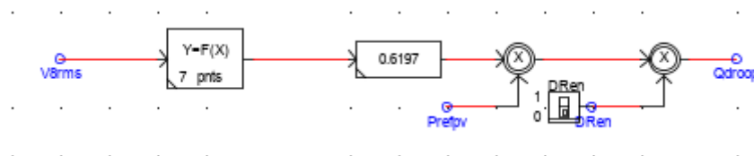
Fig. 4: Modelling of the inverter’s Voltage Droop Control
