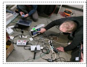
the other cabinets. The combined load was realized with LED bulbs, the laptop power adaptors and a noise generator connected to an amplifier. As expected, the combination of weak Time Dependent Impedances connected in parallel with EMC filters and a high level of non-intentional emissions, degraded significantly the performance of the PRIME PLC system.
