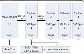
The objective of the proposed measuring campaign is to gain a better understanding of the communication process and of which parameters or type of electronic loads affect the most the communication channels for advanced PLC systems. This knowledge should help us finalizing the specification of a time variant frequency dependent grid impedance standard to be developed in the frame of the Z-NET project.
