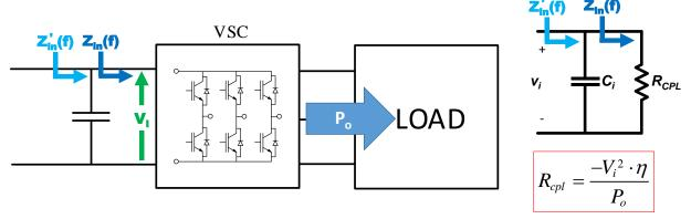
Therefore, the total impedance of the converter Zin'(s) can be obtained from the parallel of the negative resistor and the input capacitor of the converter.
